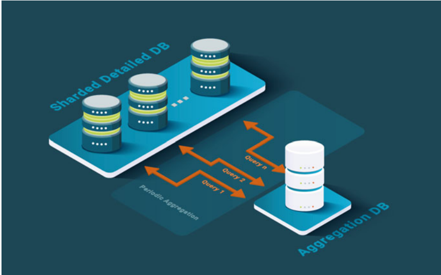
Fig. 3.7 Detail-aggregate view splitting architectural pattern
